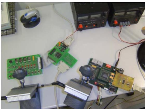
Fig. 3. Remote Control Logic of University of Deusto, web page and hardware.
