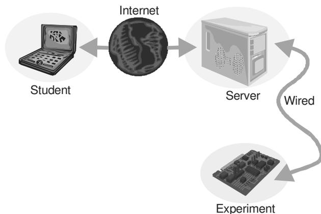
**Figure 2 Traditional Architecture of a Remote Laboratory**
