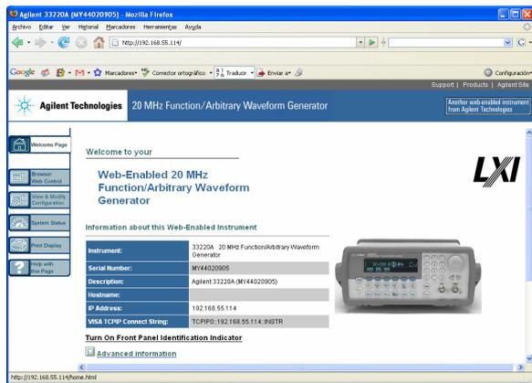
Figure 1. Browser Web Control of Agilent 33220A signal generator
