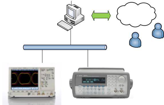
Figure 2. Remote Lab architecture based on LXI
