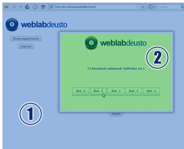
Fig. 3. “1” is the WebLab code, implemented in AJAX, and “2” is the Experiment code, implemented in Java in this case.
