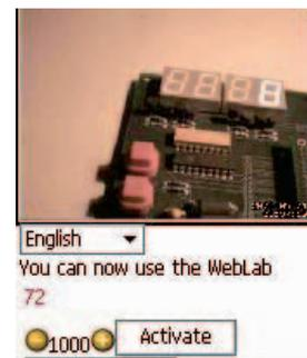
Figure 5. WebLab-Deusto 2.0 running under a Nokia 6630 device with Opera Mobile
