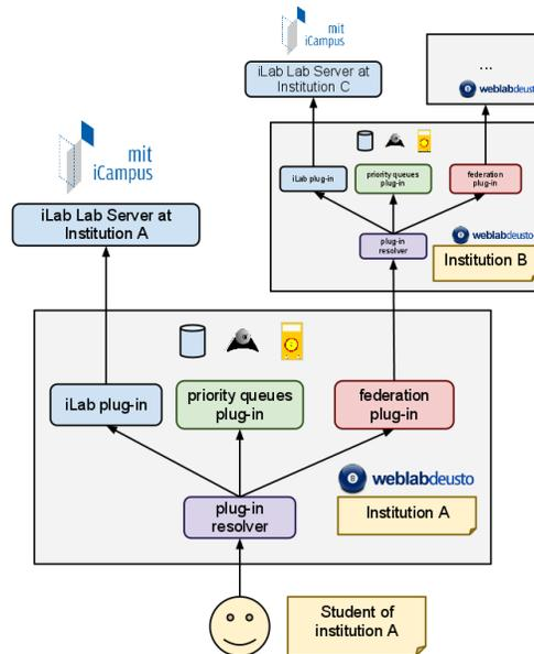
Fig. 3. Architectural overview of the iLab on WebLab-Deusto integration
