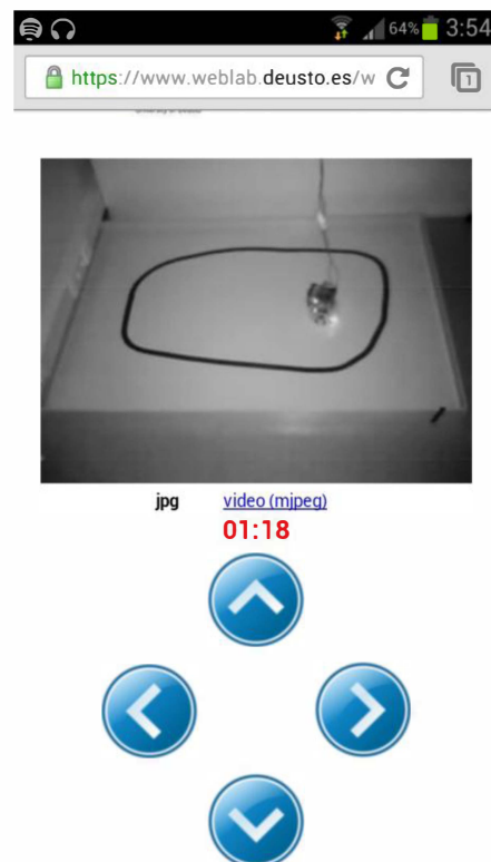
Figure 3. One of WebLab-Deusto robotics experiments (on a mobile phone, at night, video stream provided by an infrared camera).
