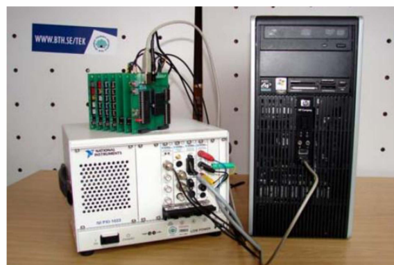
Figure 1. VISIR's hardware and equipment server. Through this means, circuits are physically built through the use of relays. [5]
