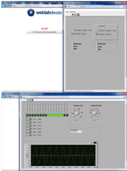
Figure 1 LabVIEW application running in WebLab-Deusto
