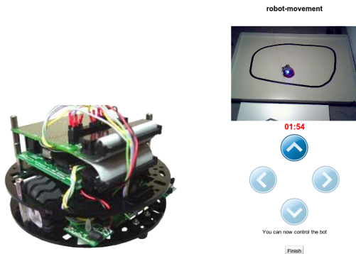
Fig. 1. Robot laboratory [1]. At the left, the mobile robot itself. At the right, the user interface once the program has been submitted.
