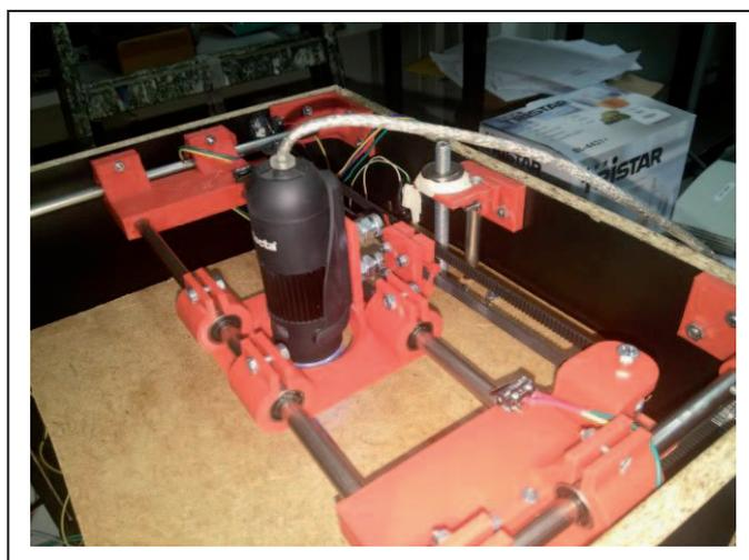
The developed prototype performs all the main features required for remotely control the microscope system:
