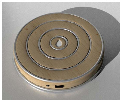
Fig. 2. First 3D render of the IC. The black rectangle on the side is the mode selector to change the feedback provided by the IC.
